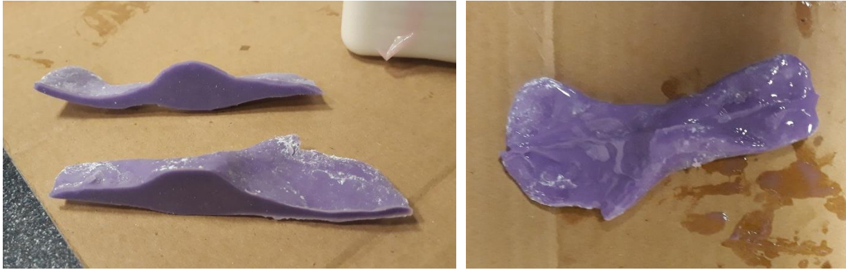
Figure 4.27. Palmar Pressure Distributor v2. The two silicone halves are united using more silicone to create the second iteration of the PPD.
