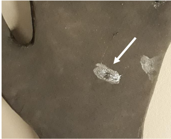
Figure 4.21. Torn Neoprene Amendment. The neoprene was a little teared in the middle of the palm of the glove. A neoprene cement layer was applied to it to avoid its expansion and final breakage.
