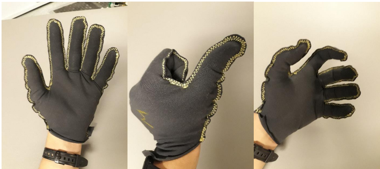
Figure 4.13. Elastic Restrain Layer v1 donned. The overlapping seam can be seen on the contour in yellow, as a Kevlar based thread was used.
