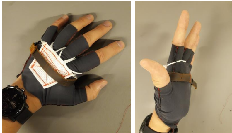
Figure 4.31. Anchoring Gauntlet v1. The inelastic white fabric can be seen sewed on the reverse side of the gauntlet, with the interdigital restraints already donned between the fingers. The brown leather belt restrain can be also appreciated in the image. The right image shows how the profile of the system looks like when the PPD is incorporated.
