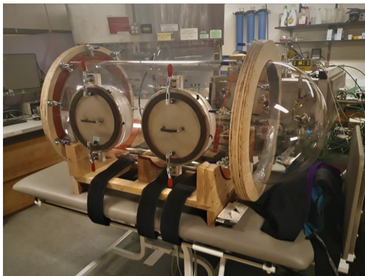
Figure 3.1. The CU Boulder Bioastronautics Glovebox. used in this study and capable of lowering its internal pressure down to -8.3 psi without appreciable leaking.
