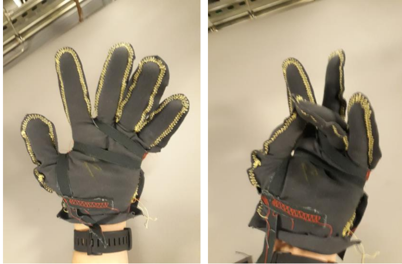
Figure 4.29. Anchoring Gauntlet Preliminary Study Concept. In the left image, the three restraints can be seen over the hand, sewed to the external gauntlet (with red thread). On the right, proof that they allow good finger and palmar movement.
