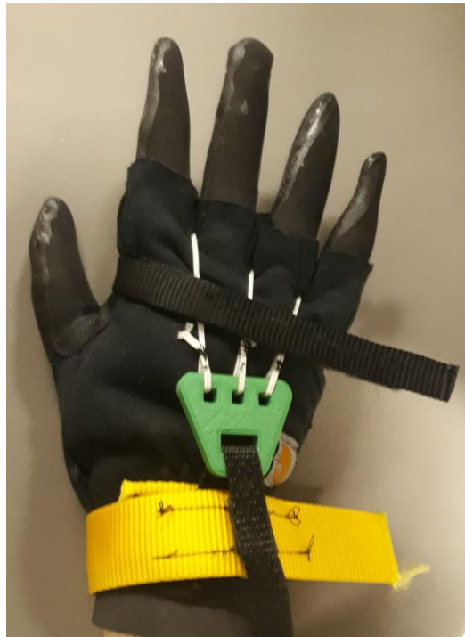
Figure 4.36. Final MCP Glove design. The three subsystems (ERL, PPD, and AG) have been integrated in this final version of the MCP Glove.
